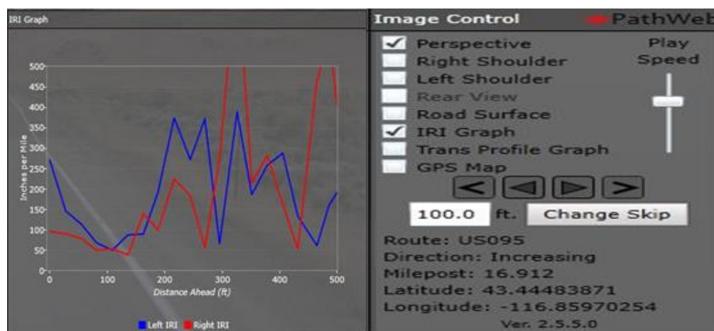
Figure 3.12 Photograph Showing Pathweb (a) IRI Graph (b) Image Control
